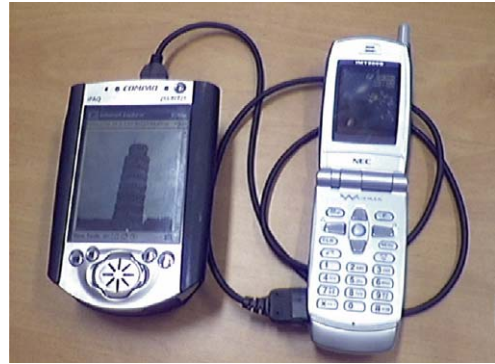
Fig. 11. Experimental test-bed (left) and PDA connected to the customization server through a UMTS terminal (right).
