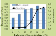
Figure 4. Influence of silica fume replacement on the grout viscosity and yield stress
