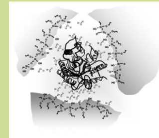
Fig. 1 – Sol-gel encapsulated enzyme.
