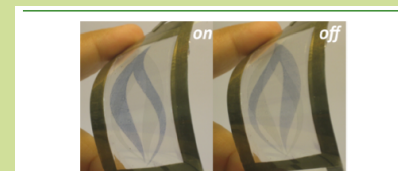
Figure 13. Photos of a flexible electrochromic device built with the tungsten oxide printed films on PET/ITO in on/off states.
