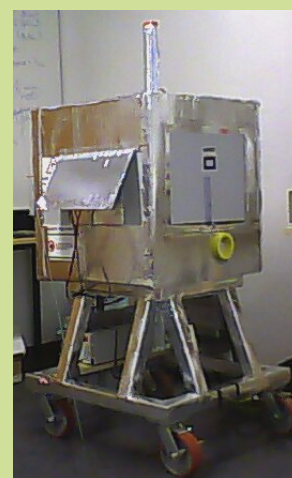
New B=0.9T NMR magnet installed in the DEC, for research with fluids in heterogeneous matrices. Permanent magnet bonus: no cryogen costs.
