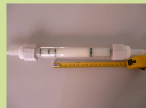
Flow cell filled with packed glass spheres, which was placed inside the magnet depicted above, to measure dispersivity with flow of water through the packing.
