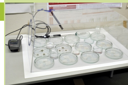
Paper samples in high humidity chamber simulating inadequate storage conditions.
