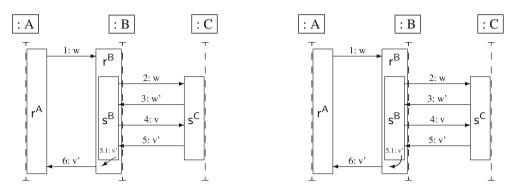
Fig. 17. SD for communication pattern: using a subsession
