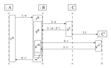
Fig. 18. SD for communication pattern: using subsessions and continuations
