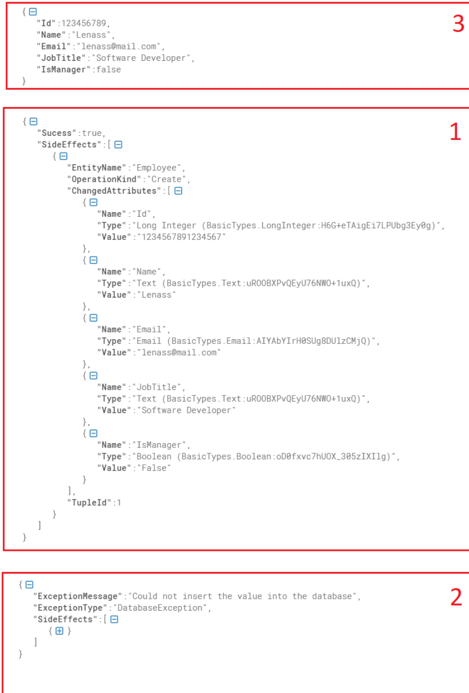
Figure 5.4: JSONs produced (boxes 1 and 2) by the execution of the AddNewEmployee Server Action (using a REST API call with the input shown in box 3) after the transformations performed by the OLP tool (presented in Figure 5.2).
