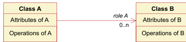
Figure 6.1: Class structure and associations between classes
