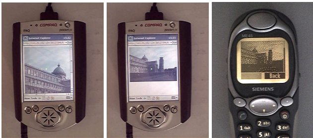
Fig. 6 – Examples: (a) image not customized to the Pocket PC display resolution (only part of the image is seen); (b) image customized to the Pocket PC display resolution; (c) image customized for a black and white WAP terminal.
