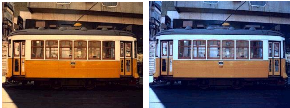
Fig. 1 – Picture with (a) sunset illumination ( T = 2,627 K) and with (b) day light illumination ( T = 8,640 K).
