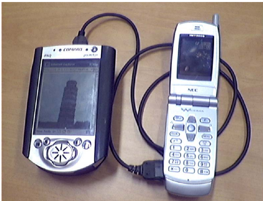
Figure 7.11 – Compaq IPAQ terminal connected to a UMTS terminal.
