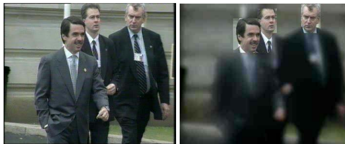
Figure 3.16 – Example of image transcoding using Importance Hint information to preserve the fidelity of the face regions.
