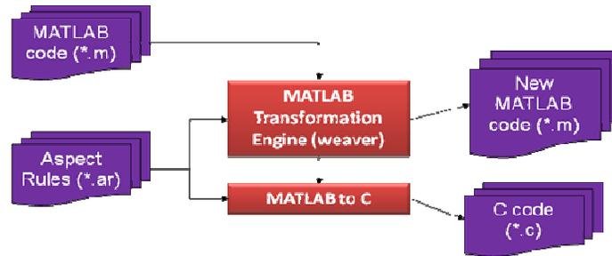
Figure 1. Outline of the MATLAB-based system augmented with aspect rules (rectangular boxes represent the two main concepts in the environment: the MATLAB weaving to produce MATLAB and C code).
